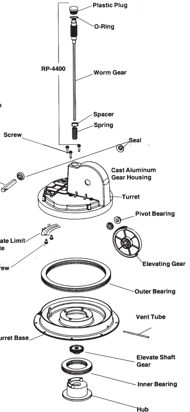
**Cutaway view of mount/gear housing**
