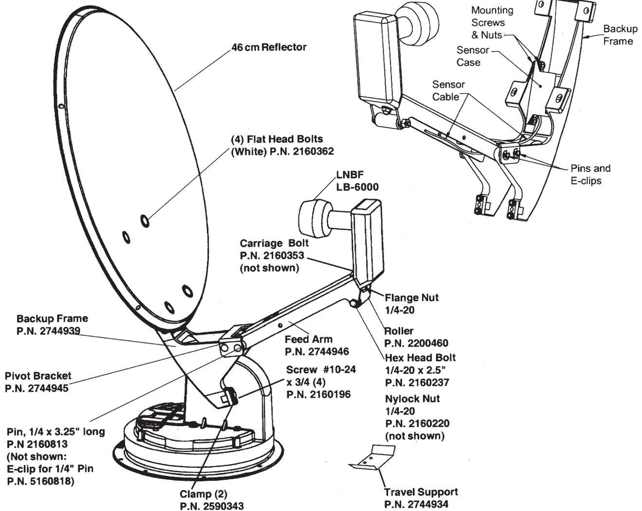
Sensor parts w/cable, installed at factory
