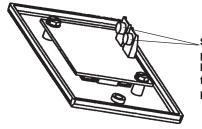
Snap battery in place, making sure battery terminals are firmly seated on wall plate terminals.
