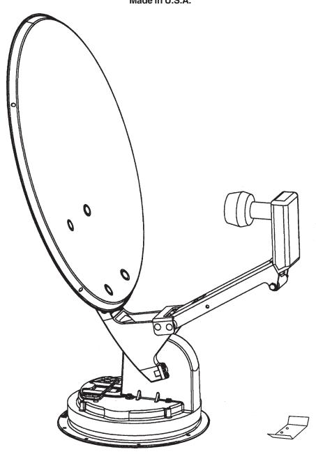
**STEP 1.** The more accurately you determine North, the easier it is to locate the satellite. Step outside and away from your vehicle. (Standing to near your vehicle can give incorrect compass readings.) It is helpful if there is a landmark on the horizon to represent North. Return to the vehicle and point the Directional Dial North, or to the landmark.
