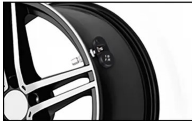
2. Install built-in sensors one by one
